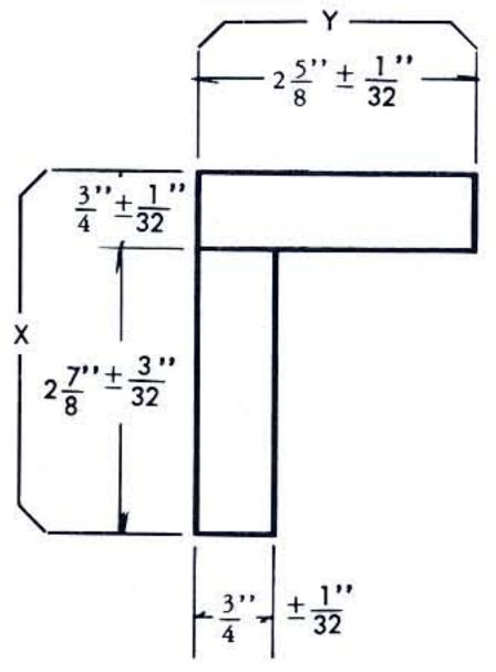
X MUST BE 3-1/2" MIN; 3-3/4" MAX. Y MUST BE 2-19/32" MIN; 2-21/32" MAX.
