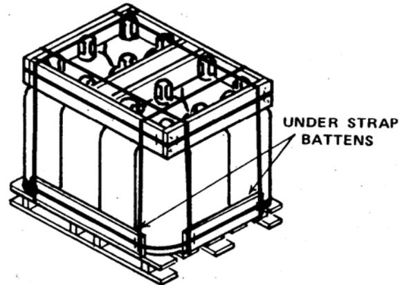
FIGURE 14. Load type IX (unstrapped and strapped) (see 5.2.9, 5.4.11.3, and 5.4.12).
