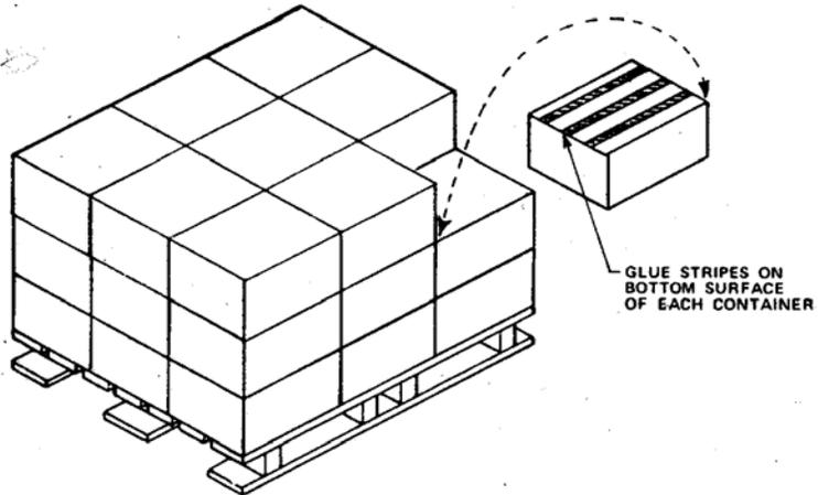
FIGURE 27. Bonding method A (glue stripes) (see 5.3.1.1).
