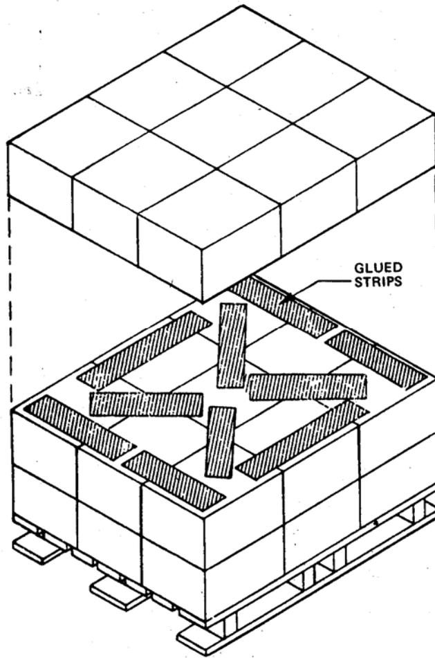
FIGURE 28. Bonding method B (glued strips) (see 5.3.1.2).
