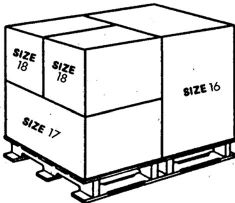
FIGURE C-6. Unit load arrangement for standard exterior containers Nos. 16, 17, and 18 (mixed sizes) (see C.6.3).
