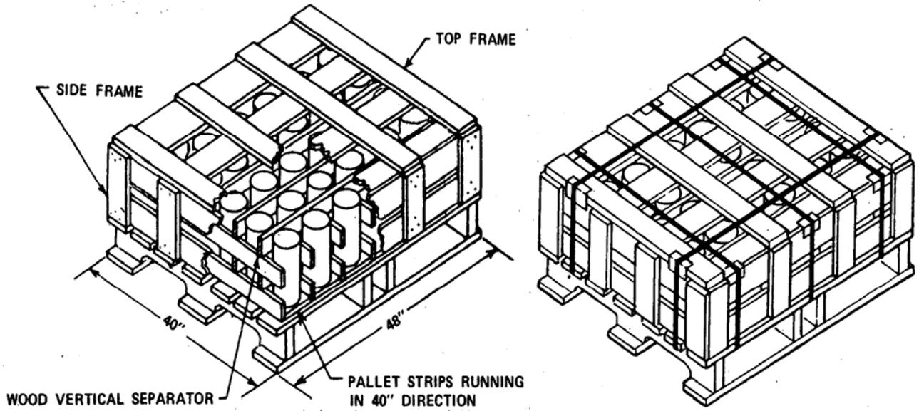
FIGURE 15. Load type X (unstrapped and strapped) (see 5.2.10).
