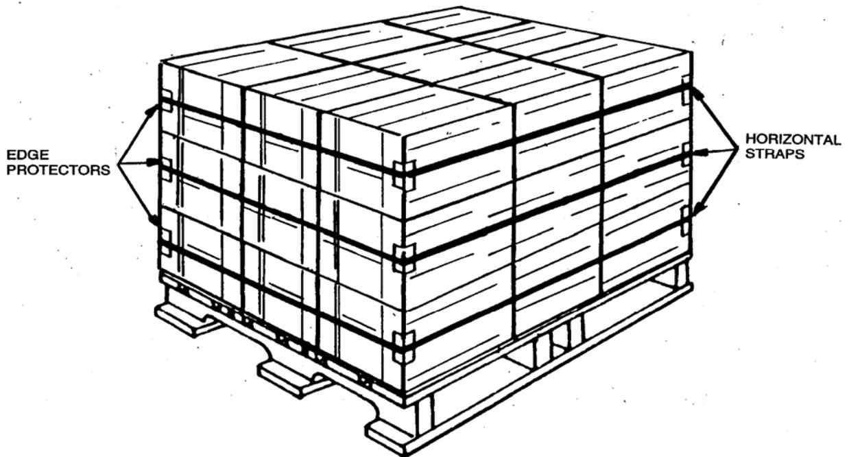
FIGURE 30. Bonding method C (each layer) (see 5.3.3.1).
