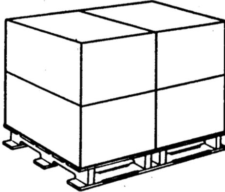
FIGURE C-3. Unit load arrangement for standard exterior container No. 17 (same size)
