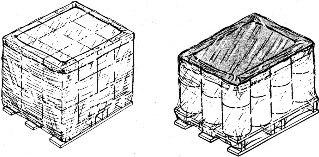
FIGURE 39. Bonding method G (stretch wrap) (see 5.3.4.2).
