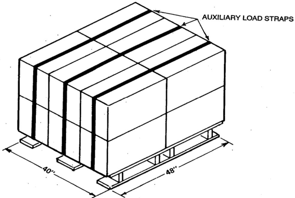
FIGURE 37. Bonding method E (auxiliary straps) (see 5.3.3.3).
