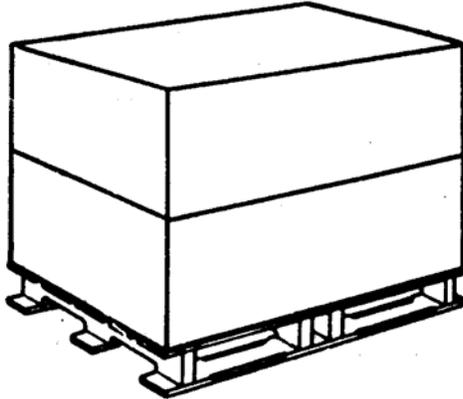
FIGURE C-1. Unit load arrangement for standard exterior container No. 15 (same size)
