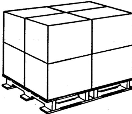
FIGURE C-4. Unit load arrangement for standard exterior container No. 18 (same size)
