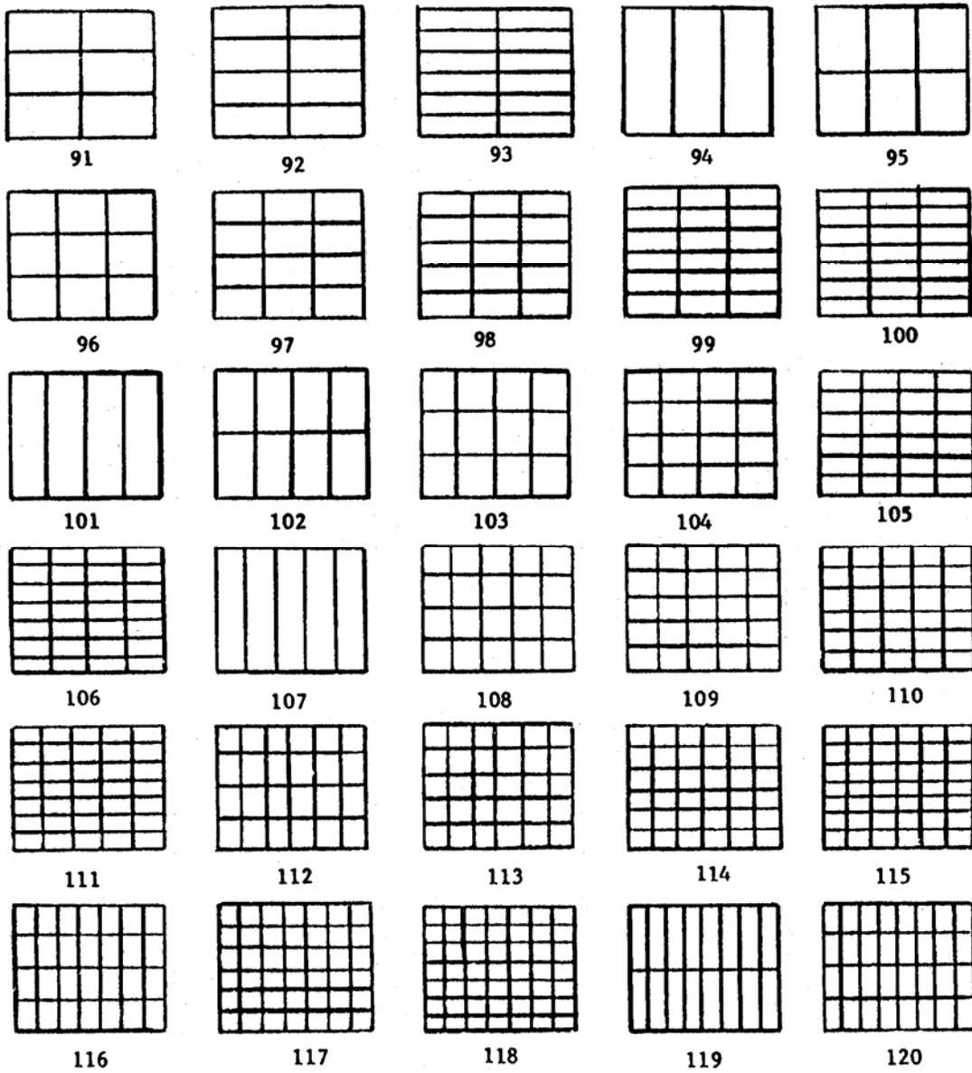
FIGURE B-1. Load patterns on 40- by 48-inch pallets (see A.2.2) (continued).
