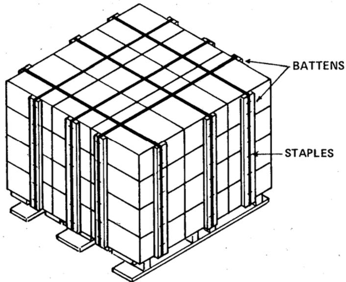
FIGURE 48. Stability dunnage type 20 (cross-strap batten) (see 5.4.11.1).
