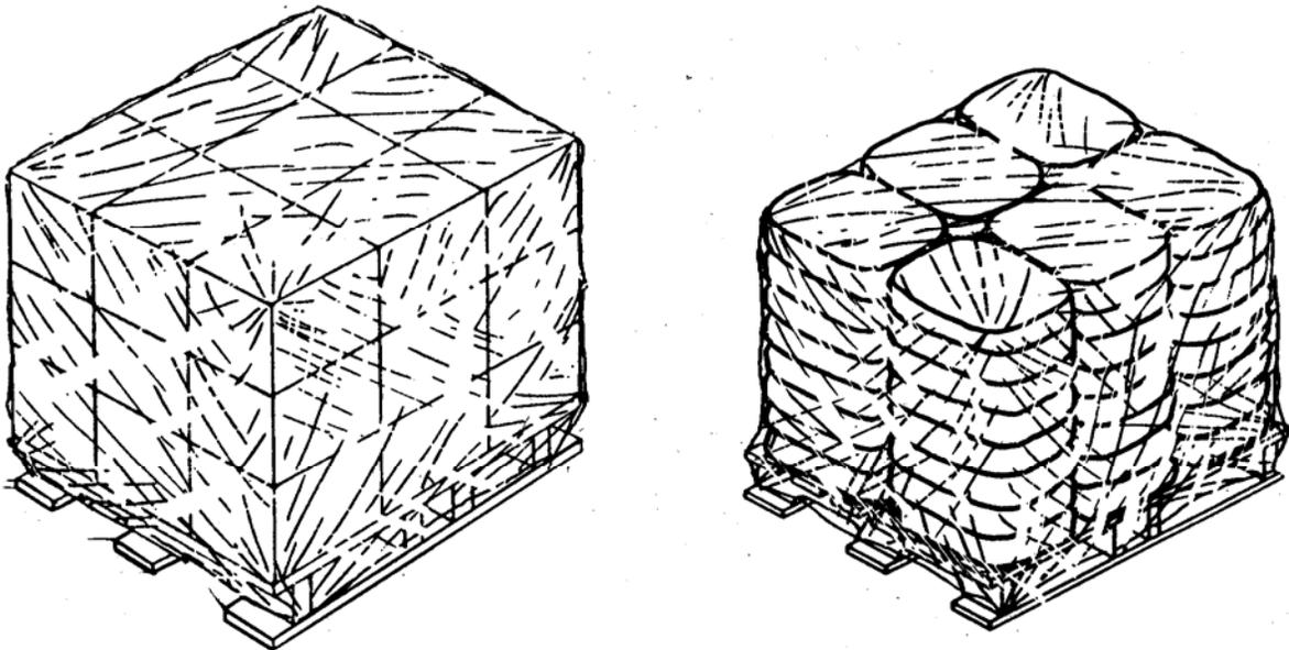
FIGURE 38. Bonding method F (shrink wrap) (see 5.3.4.1).
