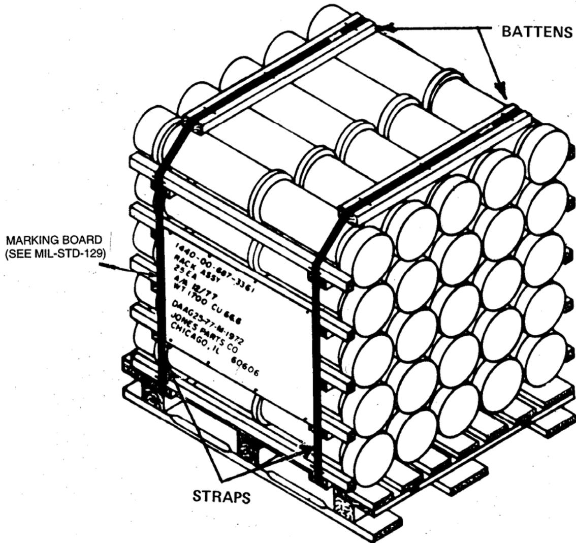
FIGURE 49. Stability dunnage type 21 (battens under- or over-the-load) (see 5.4.11.2).
